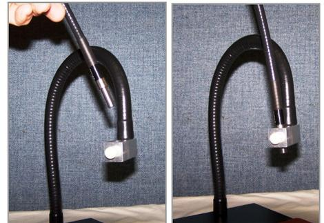
Figure 2. Insert Lightguide into Lightguide Holder
