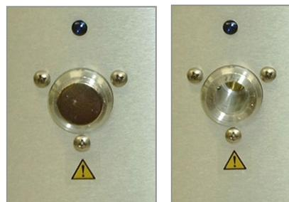
Figure 1. Lightguide Holder with protective cover and without
