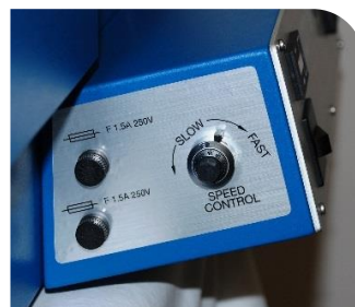
Figure 28. Conveyor Control Panel, Side
