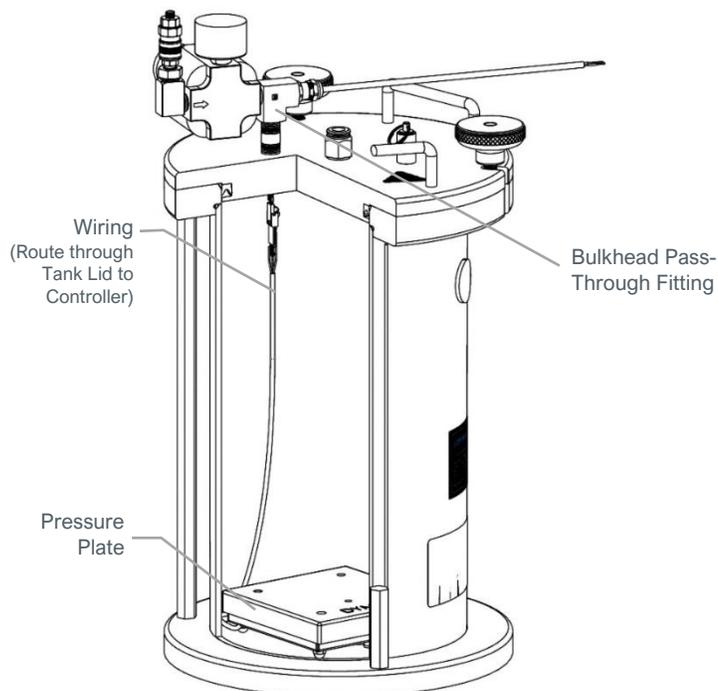
3. Strip the 1/4" wire ends and secure the connections to the SB-100 Controller. Ensure the Pressure Plate Sensor Connections are secure. (See SB-100 Controller Setup, page 17)
