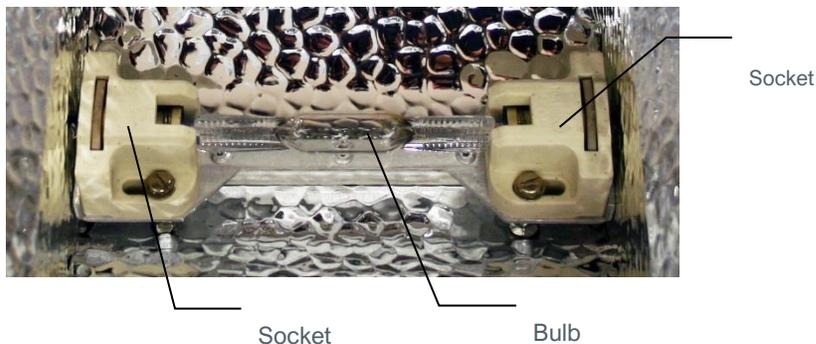
Step 5. Lightly push the Bulb toward the Socket on the opposite end of the lamp so that the end being grasped can be lifted clear of the Socket.
