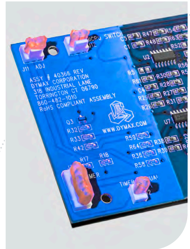
Maskants can be used to prevent coatings from covering or flowing under components
