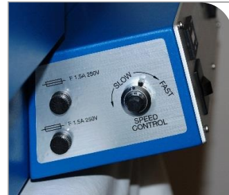
Figure 28. Conveyor Control Panel, Side
