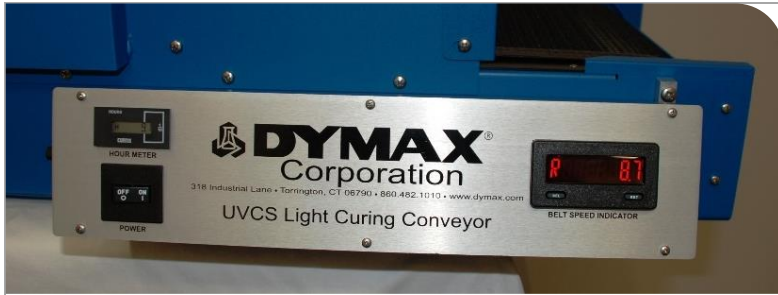
Figure 27. Conveyor Control Panel, Front
