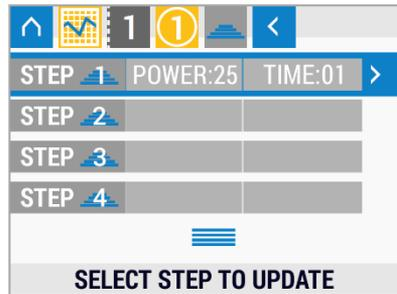
On the steps menu (Figure 20), the user can see the power and time settings for each step. To edit the step, navigate using the up and down buttons, then Right button to edit.
