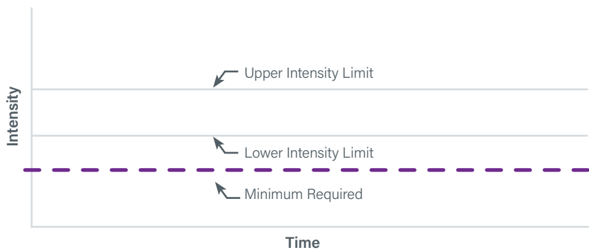
Figure 2. A Controlled UV Spot-Curing Process
