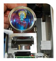
Figure 4. Remove Bulb from Bulb Mount
