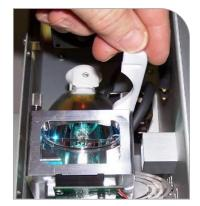
Figure 3. Lift Bulb Mounting Bracket
