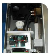
Figure 2. Bulb Installed in Bulb Mount
