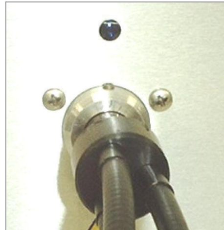
Figure 11. Bulb Status Indicator Light
