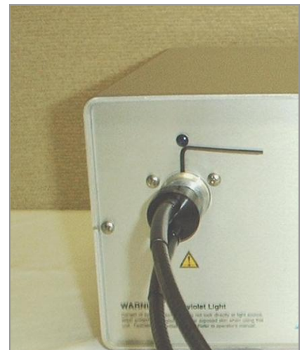
Figure 6. Insert Lightguide into Lightguide Mount
