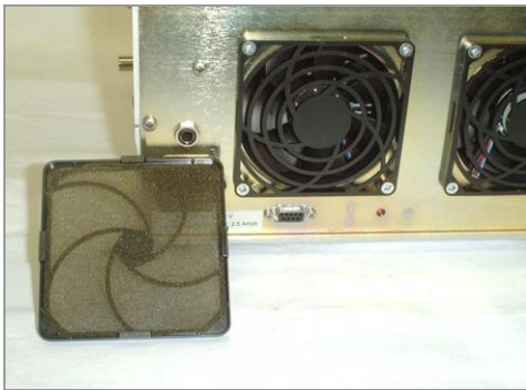
Figure 13. Exhaust Fans with Fan Filters Removed
