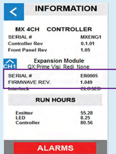
Figure 36. System Information Screen Identifying MX-4E
