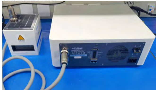
Figure 7. Interconnect Cable Installed
