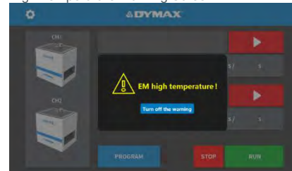
Figure 38. High Temperature Warning Screen
