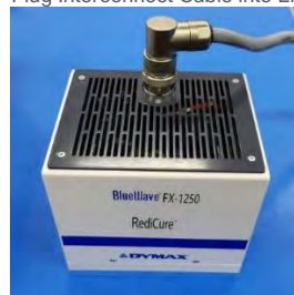
Figure 13. Plug Interconnect Cable into Emitter
