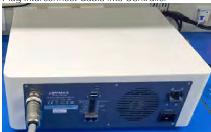
Figure 12. Plug Interconnect Cable into Controller
