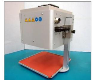
Figure 6. Attach Reflector to Mounting Stand
