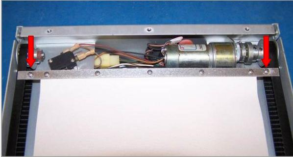
Figure 7. Loosen End Screws
