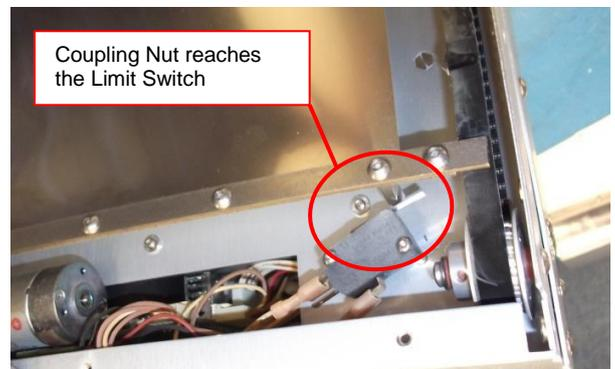
Figure 12. Rear Limit Switch
