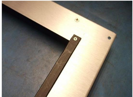
Figure 16. Install M3 x 6 mm Screws into Wear Strip
