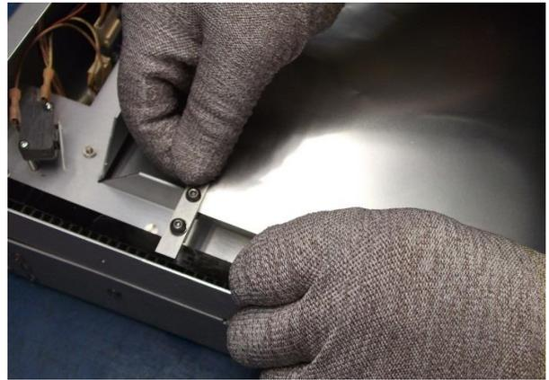
Figure 10. Slide the Clamp Bar onto the Belt
