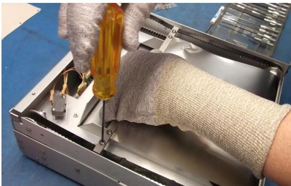
Figure 11. Tighten the M4 x 6 mm End Screws
