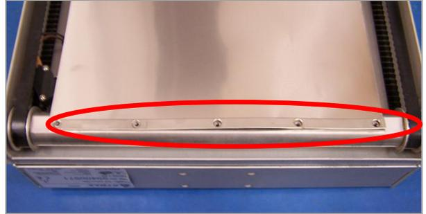
Figure 8. Five Retaining Screws
