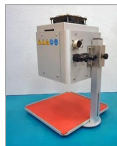
Figure 7. Attach Reflector to Mounting Stand
