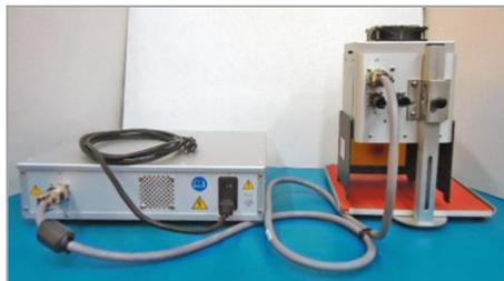
Figure 9. Connect Power Supply to Reflector
