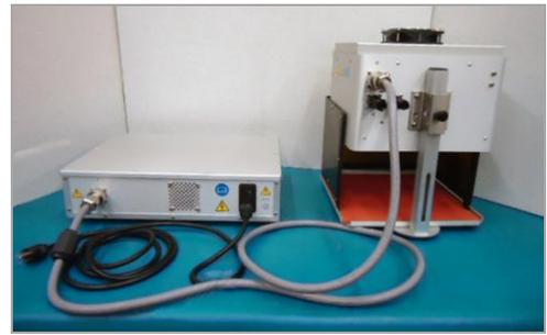
Figure 8. Connect Power Supply to Reflector
