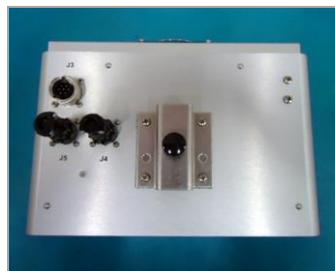
Figure 5. Reflector Mounting Bracket & Bypass Connectors Installed
