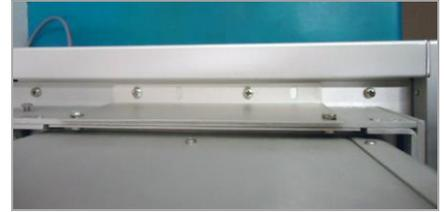
Figure 5. Attach Securing Bracket with M4 x 8 mm screws
